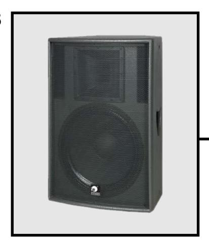
IE-15 and IE-215 series are the high performance and wide-bandwidth system. Extended frequency response is provided by a 15"(380mm) / two 15"(380mm) LF driver separately, teamed with a 1.4" exit compression driver mounted on a rotatable 80°X50°constant directivity HF horn.
